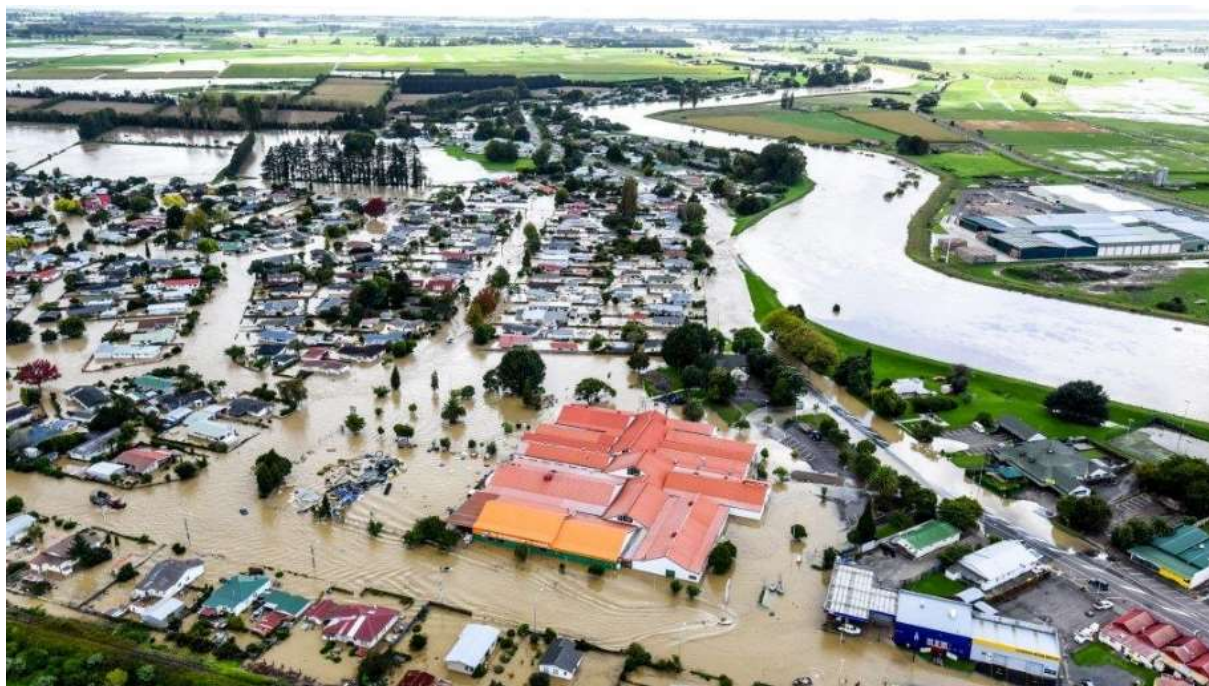
Extensive inundation of Edgumbe following the failure of Rangitāiki River stop-banks in April 2017.
