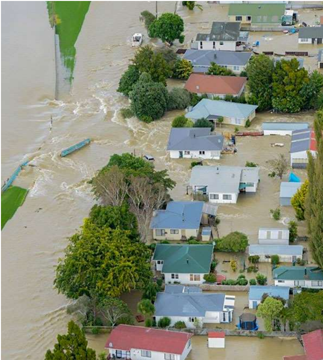
Extensive inundation of Edgecumbe following the failure of Rangitāiki River stop-banks in April 2017.
