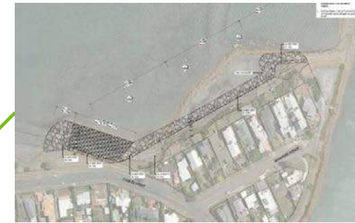
Whakarire Ave Revetment
